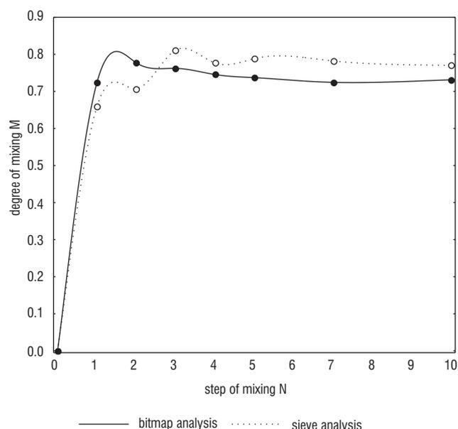
FIGURE 5. Changeability of the degrees of mixing vs. the number of steps with the RSI System.
