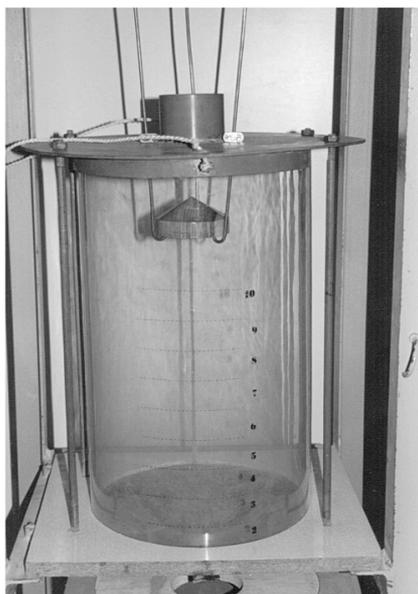
FIGURE 3. The cone situated in axes of bins – Roof Shaped Insert System.
