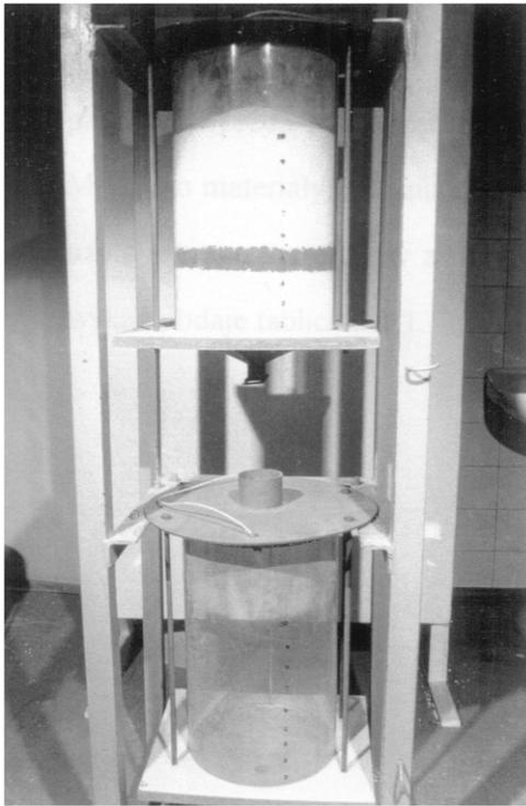
FIGURE 2. Laboratory mixing system using a funnel-flow method; a supplying bin over a receiving bin with the prepared tracer load and dispersing phase.
