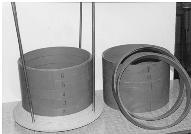
FIGURE 1. Dismantling analytical bin as equivalent to geometric dimensions of laboratory bins employed in the mixing process using a funnel-flow method.
