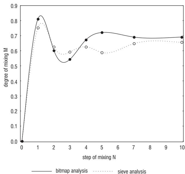
FIGURE 4. Changeability of the degrees of mixing vs. the number of steps without the RSI System.
