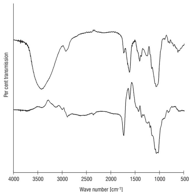
FIGURE 3. Differential spectrum of the xanthan gum-ovalbumin complex prepared by electrosynthesis from the 1:1 mixture of components from which the spectrum of ovalbumin was subtracted (below). The spectrum of xanthan gum (above) is quoted for comparison. The spectrum for analogous complex prepared by coacervation was identical.
