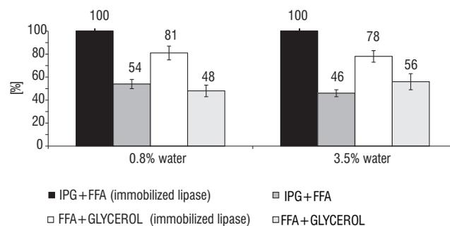
FIGURE 7. Conversion to protected MAG and synthesis yield of MAG by lipase from *Candida antarctica*.
