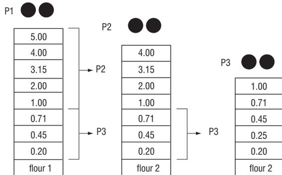
FIGURE 1. The milling diagram used (dimensions of sieves in mm): P1, P2, P3 – the first, the second and the third stage.
