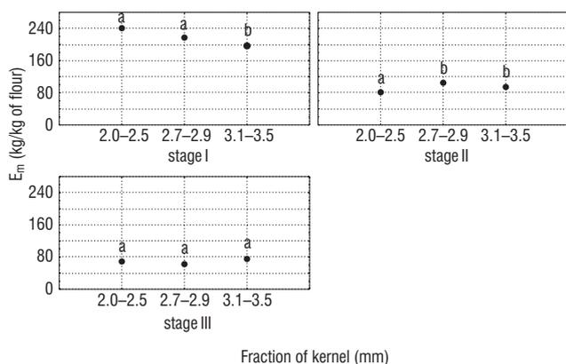
FIGURE 7. The influence of kernel size on grinding index ( $E_m$ ) for individual grinding stages (values designated by the different letters are significantly different,  $\alpha = 0.05$ ).
