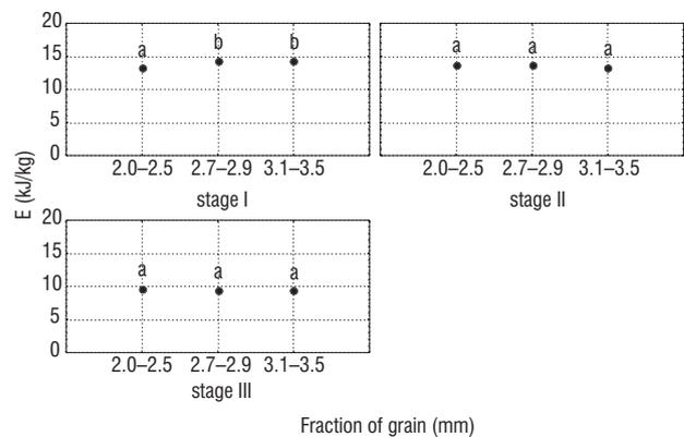
FIGURE 5. The influence of kernel size on specific milling energy (E) for individual grinding stages (values designated by different letters are significantly different,  $\alpha = 0.05$ ).
