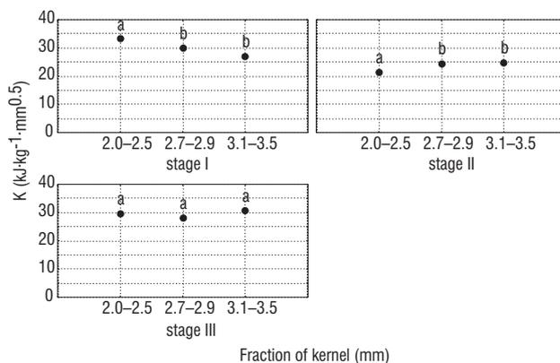
FIGURE 8. The influence of kernel size on grinding index (K) for individual grinding stages (values designated by the different letters are significantly different,  $\alpha = 0.05$ ).
