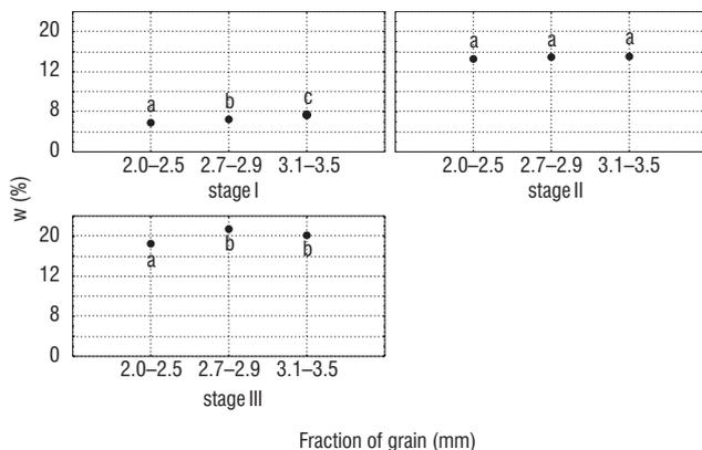
FIGURE 3. The influence of kernel size on flour yield (w) for respective grinding stages (values designated by the different letters are significantly different,  $\alpha = 0.05$ ).
