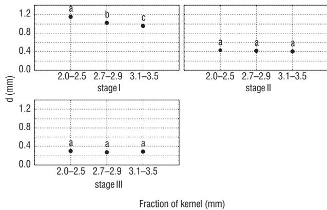
FIGURE 2. The influence of kernel size on the average particle size of ground material (d) for respective grinding stages (values designated by the different letters are significantly different,  $\alpha = 0.05$ ).
