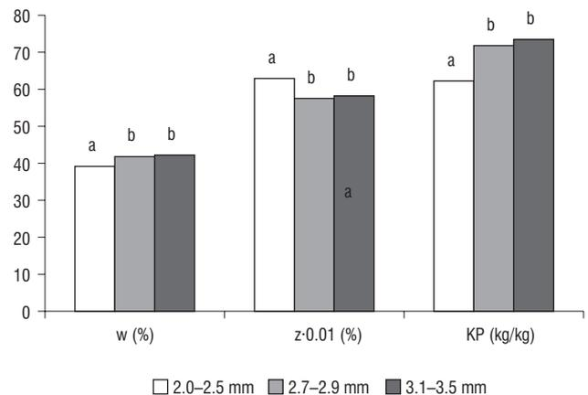
FIGURE 4. The influence of kernel size on the total flour yield (w), ash content (z) and milling efficiency index (KP) (values designated by the different letters are significantly different,  $\alpha = 0.05$ ).
