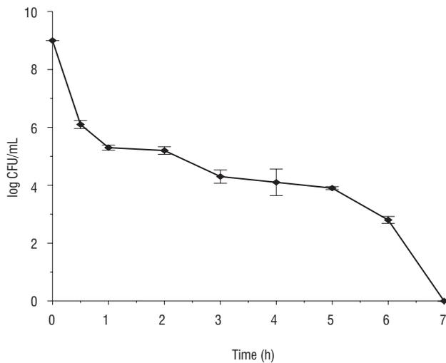
FIGURE 2. The effect of pressurization time at 193 MPa and  $-20^{\circ}\text{C}$  on viability of *E. coli* (generating time of the pressure – 90 min).
