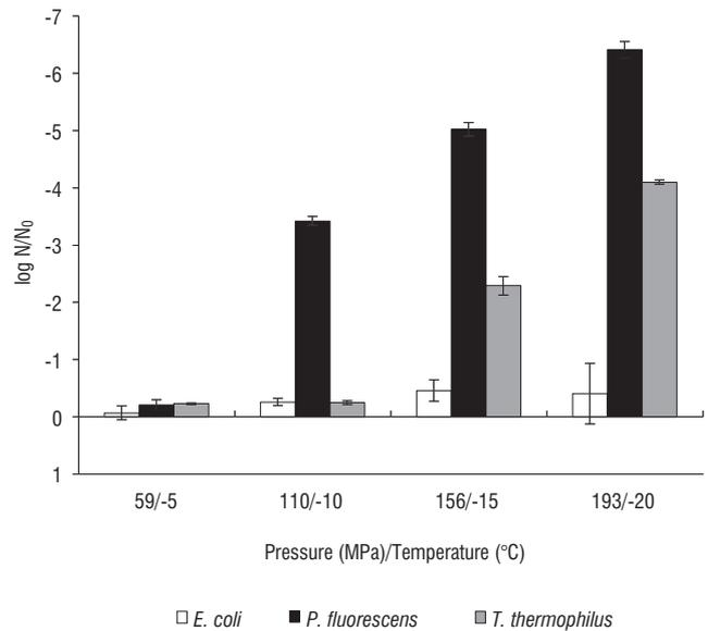
FIGURE 3. The effect of high pressure at subzero temperature on viability loss of *E. coli*, *P. fluorescens* and *T. thermophilus* (during 40 min generating of the pressure). <sup>1</sup>) N – the number of cells detected after pressurization; N<sub>0</sub> – the number of cells in the control.
