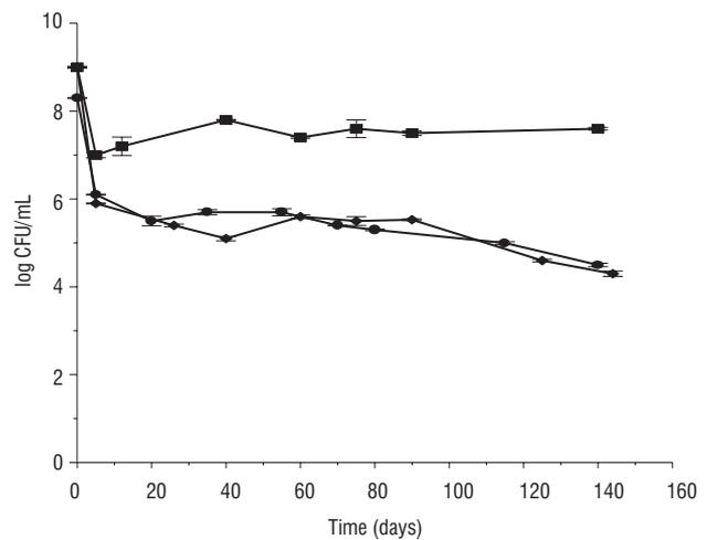
FIGURE 4. The effect of storage at  $-20^{\circ}\text{C}$  under atmospheric pressure on viability loss of *E. coli* ( $\blacklozenge$ ), *P. fluorescens* ( $\bullet$ ) and *T. thermophilus* ( $\blacksquare$ ).
