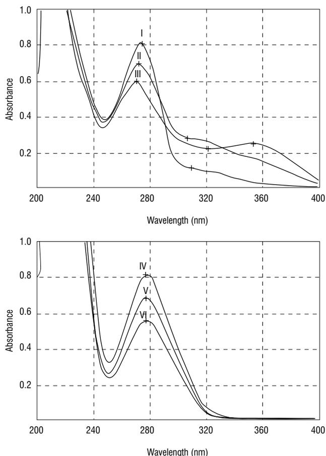
FIGURE 2. UV spectra of fractions separated on a Toyopearl HW-40S column with ethanol as mobile phase.
