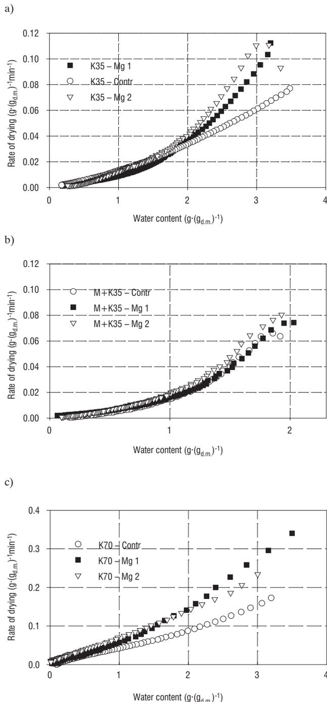
FIGURE 1. Relationship between the rate of drying and water content in yeast biomass under different drying conditions: a) variant K35, b) variant M+K35, c) variant K70.
