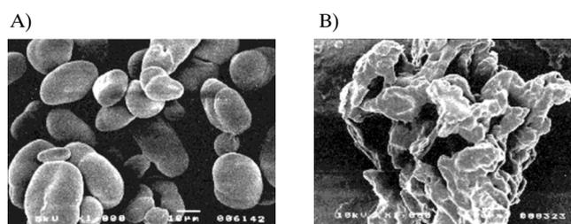
FIGURE 3. SEM-microstructure of native pea starch (A) and its preparation (B).
