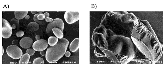
FIGURE 2. SEM-microstructure of native potato starch (A) and its preparation (B).
