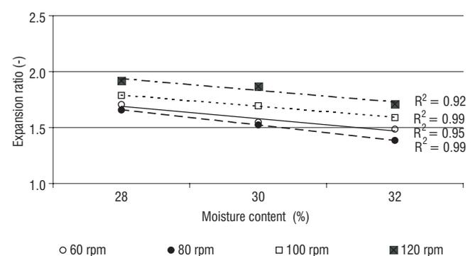
FIGURE 1. The expansion ratio of pasta processed with different moisture content of dough from a flour type 450 and 2% of salt under various extrusion screw speed.
