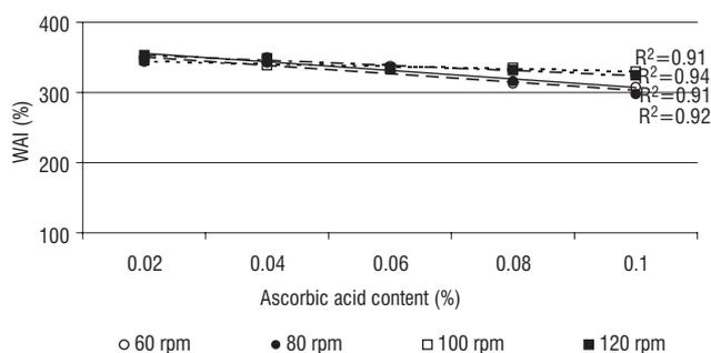
FIGURE 2. Water absorption index for pasta products processed from a flour type 550 with ascorbic acid addition (30% m.c.) at various extrusion screw speed.
