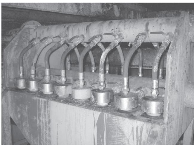
FIGURE 3. The battery of hydrocyclones in MZ-technology.
