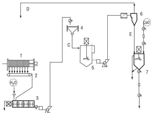
FIGURE 2. Simplified scheme of MZ-method at sugar factory Vrdu. Legend: 1 – filter press, 2 – mud conveyor, 3,5 – mixers, 4 – sieve, 6 – hydrocyclones, 7 – reactor; C, D, E – points of suspensions sampling
