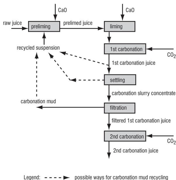
FIGURE 1. A simplified scheme of the first part of juice purification.
