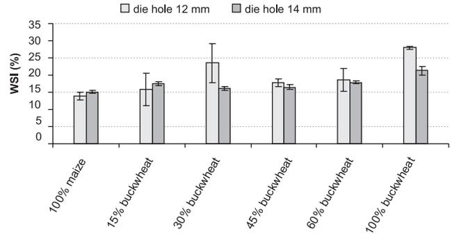
FIGURE 3. Effect of die outlet hole diameter on water solubility index (WSI) of maize-buckwheat extrudate.
