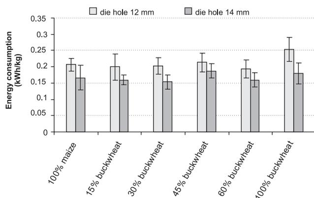
FIGURE 5. Effect of die outlet hole diameter on electrical energy consumption during extrusion of maize-buckwheat mixtures.
