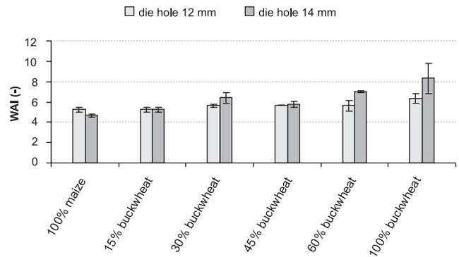
FIGURE 4. Effect of die outlet hole diameter on water absorption index (WAI) of maize-buckwheat extrudate.
