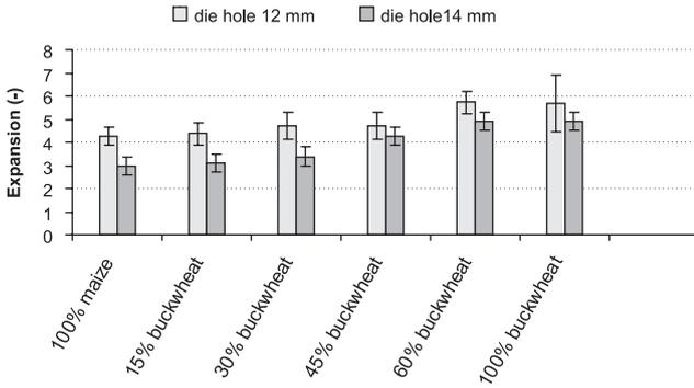
FIGURE 1. Effect of die outlet hole diameter on expansion ratio of maize-buckwheat extrudate.
