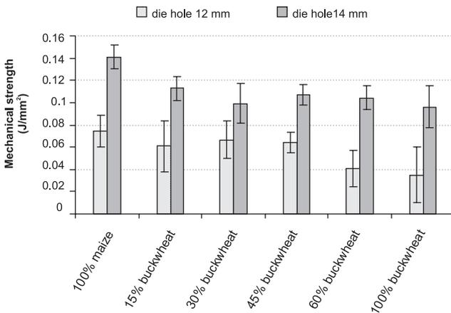
FIGURE 2. Effect of die outlet hole diameter on mechanical strength index of maize-buckwheat extrudate.
