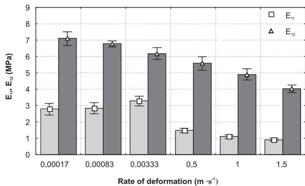
FIGURE 1. Modulus of elasticity  $E_{11}$  and  $E_{12}$  versus deformation rate of the carrot samples in the state of uniaxial stress.
