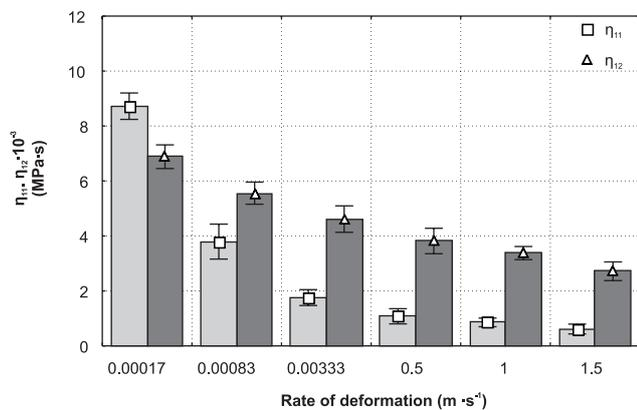
FIGURE 2. Viscosity ratios  $\eta_{11}$  and  $\eta_{12}$  versus deformation rate of the carrot samples in the state of uniaxial stress.
