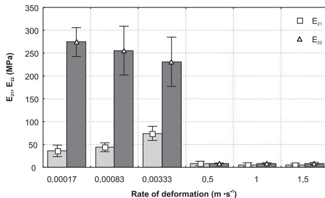
FIGURE 3. Modulus of elasticity  $E_{21}$  and  $E_{22}$  versus deformation rate of the carrot samples in the state of uniaxial strain.
