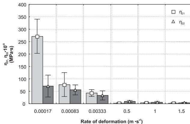
FIGURE 4. Viscosity ratios  $\eta_{21}$  and  $\eta_{22}$  versus deformation rate of the carrot samples in the state of uniaxial strain.
