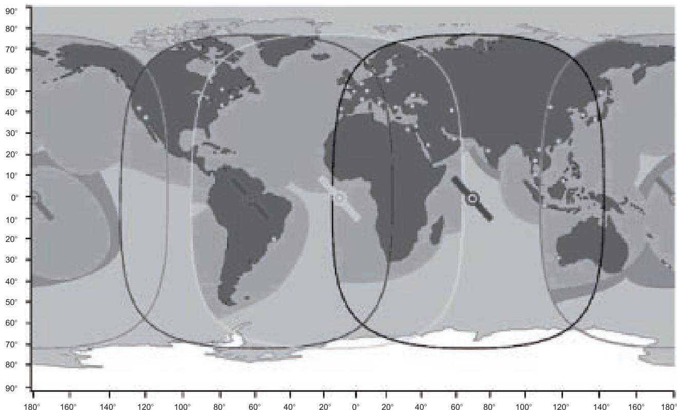
FIGURE 4. Satellite INMARSAT global range [Inmarsat, 2007].
