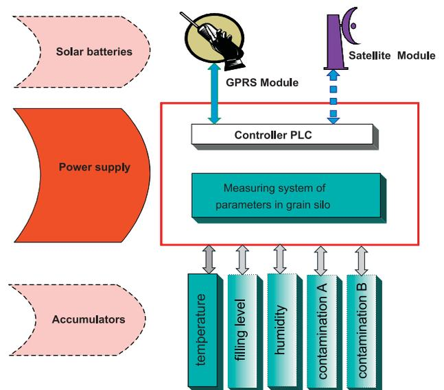
FIGURE 2. Telemetric module application used in grain silo monitoring system.
