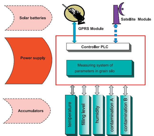
FIGURE 2. Telemetric module application used in grain silo monitoring system.
