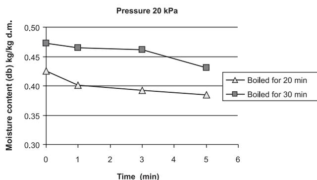
FIGURE 3. Changes in the moisture content (dry basis) of raw materials subjected to 20 and 30 min hydro-thermal treatment and next to the vacuum pressure of 20 kPa.
