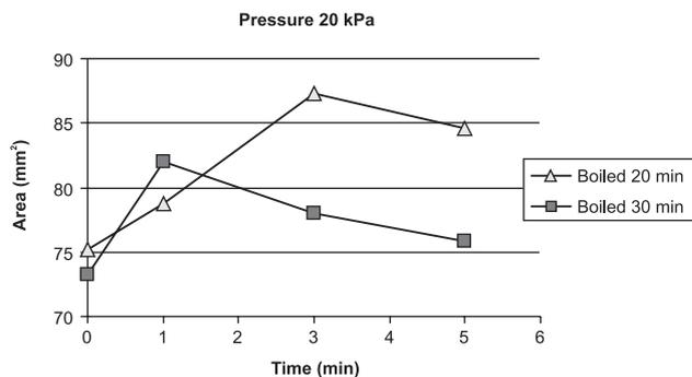
FIGURE 6. Changes in horizontal projection area for maize seeds in samples hydro-thermally treated for 20 and 30 min and subjected to 20 kPa vacuum pressure.
