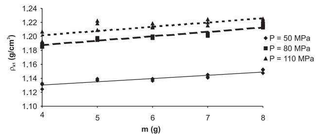
FIGURE 4. Density of the agglomerate  $\rho_{kl}$  after 24 h of storage time, in relation to the mass of compacted sample  $m$ , at different loading pressures  $P$  (at 15 mm diameter chamber).
