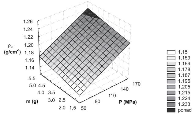
FIGURE 2. Density of the agglomerate after 24 h of storage time  $\rho_{kl}$ , in relation to the mass of compacted sample  $m$ , and loading pressure  $P$  (12 mm diameter chamber).
