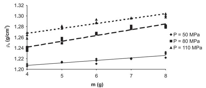
FIGURE 3. Density of the agglomerate  $\rho_k$ , in relation to the mass of compacted sample  $m$ , at different loading pressures  $P$  (15 mm diameter chamber).
