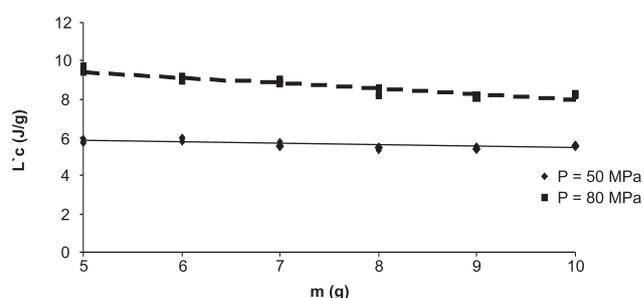
FIGURE 6. Specific compression work  $L^c$ , in relation to the mass of compacted sample  $m$ , at different loading pressures  $P$  (18 mm diameter chamber).
