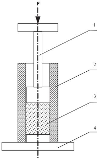
FIGURE 1. Scheme of the compression assembly: 1 – piston, 2 – cylinder, 3 – compressed material, 4 – bottom stand.
