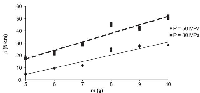
FIGURE 5. Strength of the agglomerate  $\rho$  in relation to the mass of compacted sample  $m$ , at different loading pressures  $P$  (18 mm diameter chamber).
