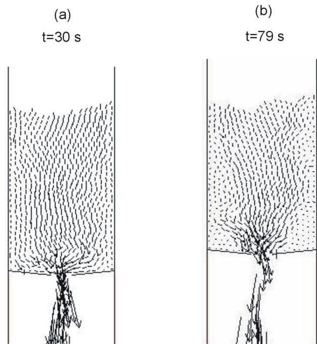
FIGURE 6. Distribution of velocities of particles for  $\mu=0.1$  (a) and  $\mu=0.7$  (b).
