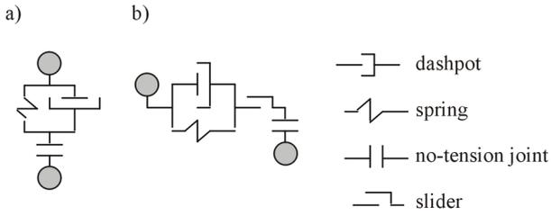
FIGURE 1. Contact model for DEM simulations in the normal (a) and tangential (b) directions.
