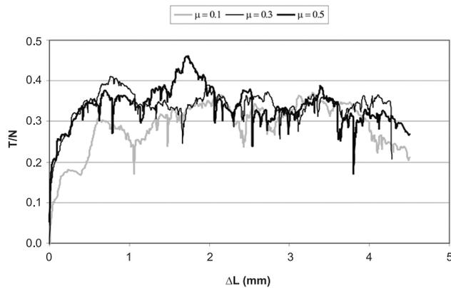
FIGURE 5. Evolution of T/N ratio versus displacement for different values of friction coefficient.
