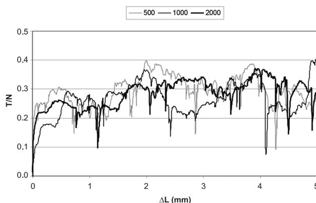
FIGURE 4. Evolution of T/N ratio versus displacement for different number of elements.
