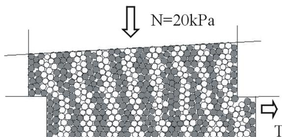
FIGURE 2. Direct shear box.
