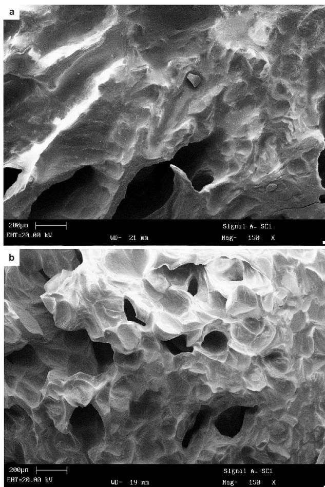
FIGURE 10. SEM pictures of French fries pre-dried with (a) vacuum microwave pre-drying method and (b) convective pre-drying method.
