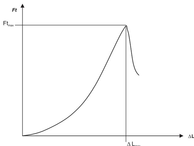
FIGURE 1. Determination of the maximum cutting force  $Ft_{max}$  (N).
