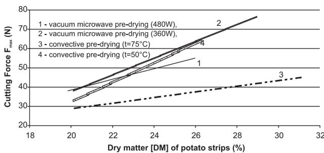
FIGURE 5. Values of the maximum cutting force ( $F_{max}$ ) of French fries as dependent on the pre-drying methods of potato strips.
