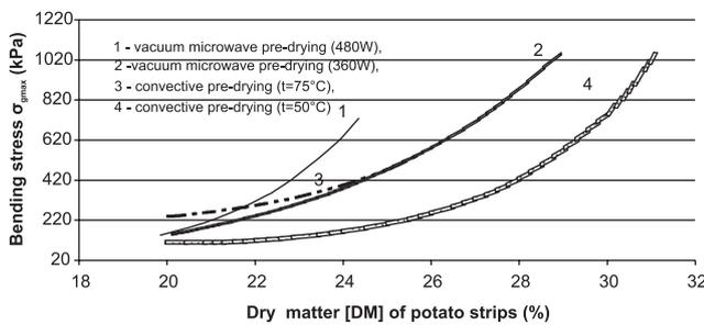
FIGURE 6. Values of the maximum bending stress ( $\sigma_{g,max}$ ) of French fries as dependent on the pre-drying methods of potato strips.
