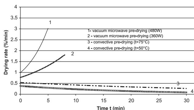
FIGURE 3. Drying rate curves of potato strips under various pre-drying methods.
