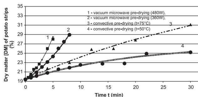
FIGURE 2. The kinetics of pre-drying potato strips with the vacuum microwave method: 1- (480W) and 2- (360W) and convection method: 3 ( $t = 75^\circ C$ ), 4 ( $t = 50^\circ C$ ).
