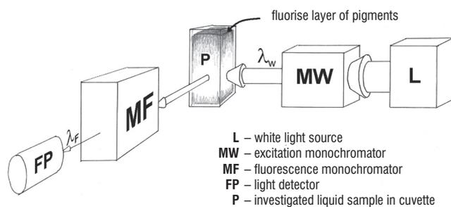
FIGURE 3. Fluorescence measurement with traditional method.
