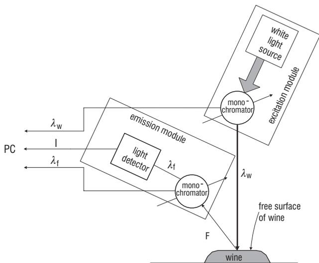
FIGURE 4. The new conception of fluorescence measuring.
