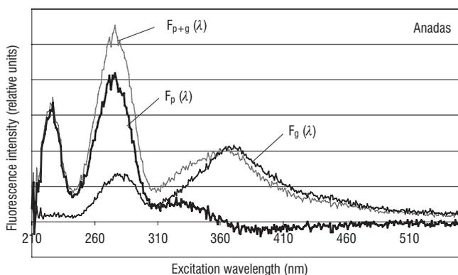
FIGURE 5. Fluorescence spectra of white wine registered above the sample surface ( $F_{p+g}(\lambda)$ ), under the surface ( $F_g(\lambda)$ ) and the calculated surface fluorescence spectrum ( $F_p(\lambda)$ ).
