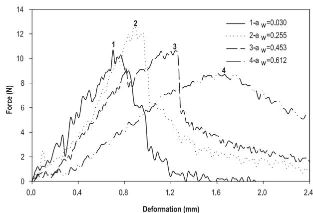
FIGURE 1. Breaking curves of rye crisp bread at different water activity.
