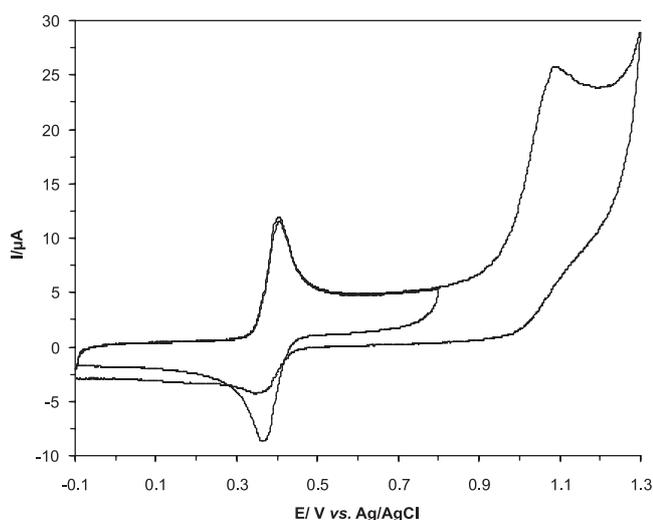
FIGURE 2. The cyclic voltammograms of 0.25 mmol/L of standard solution (final concentration) of rutin in 0.1 mol/L sodium acetate-acetic buffer (final concentration at pH 4.5) in 90% methanol recorded from -100 to +800 mV and from -100 to +1300 mV; scan rate  $100 \text{ mV s}^{-1}$ .
