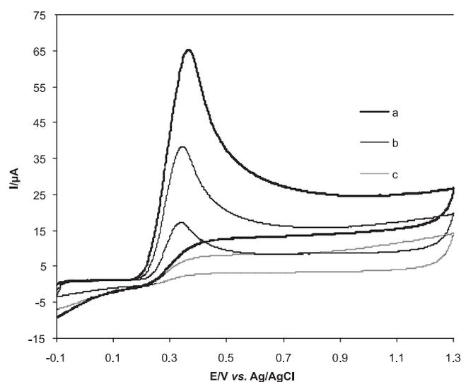
FIGURE 3. Selected cyclic voltammograms of (a) 2.5 mmol/L, (b) 1.25 mmol/L and (c) 0.5 mmol/L of Trolox solution (final concentration) in 0.1 mol/L sodium acetate-acetic buffer (final concentration at pH 4.5) in 90% methanol recorded from -100 to +1300 mV; scan rate  $100 \text{ mV s}^{-1}$ .
