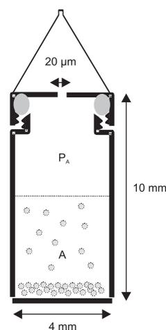
FIGURE 2. A schematic view of a Knudsen cell hanging in the thermo-balance.
