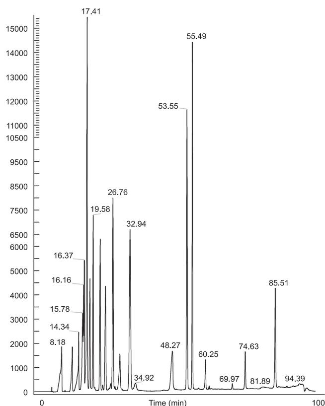
FIGURE 1. An HPLC chromatogram showing separation of twenty two standard phenolic compounds.
