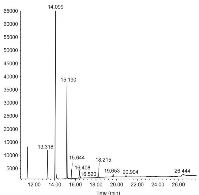
FIGURE 4. GC-MS analysis of fatty acid methyl methyl esters extracted from ber seed oil by Soxhlet procedure.
