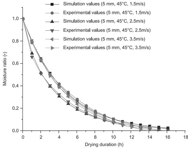
FIGURE 4. The influence of hot air velocity on MR. Comparison between the values of the Page model and the experimental data at different hot air velocity (hot air temperature at 45°C, fillet thickness at 5 mm).
