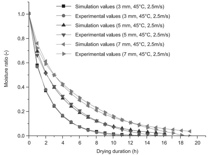
FIGURE 6. The influence of fillet thickness on MR. Comparison between the values of the Page model and the experimental data at different thickness of tilapia fillets (hot air temperature at 45°C, hot air velocity at 2.5 m/s).
