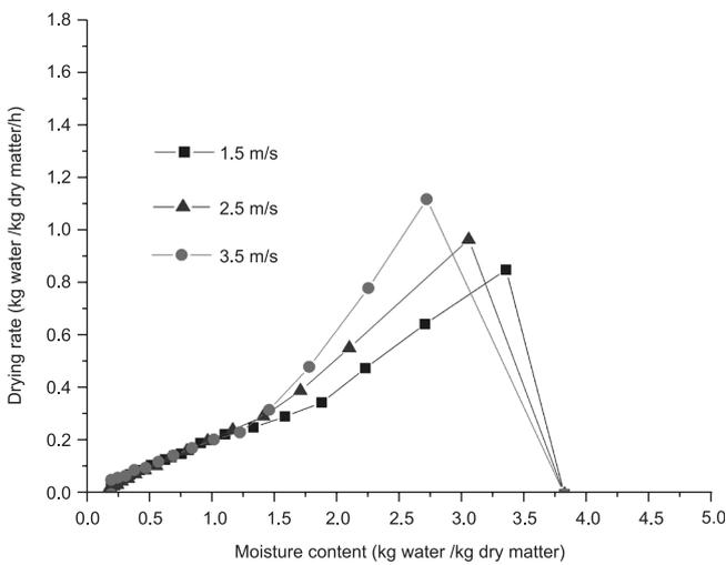
FIGURE 5. The influence of hot air velocity on drying rate (hot air temperature at 45°C, fillet thickness at 5 mm).
