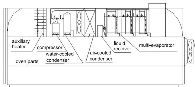
FIGURE 1. The schematic of the heat pump dryer.
