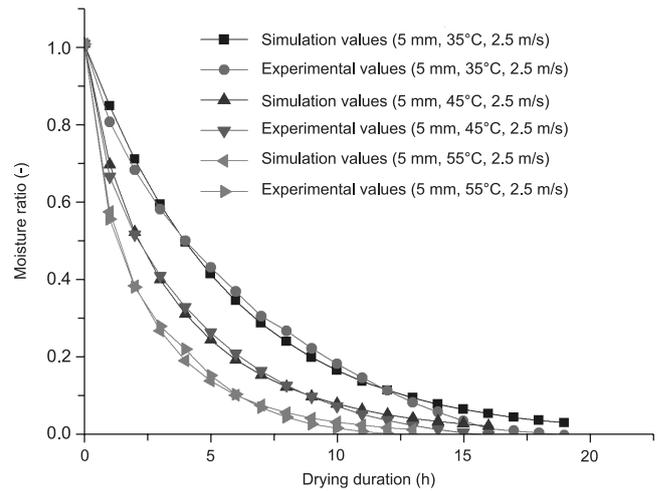
FIGURE 2. The influence of the temperature of hot air on  $MR$ . Comparison between the values of the Page model and the experimental data at different drying temperatures (hot air wind speed at 2.5 m/s, fillet thickness at 5 mm).
