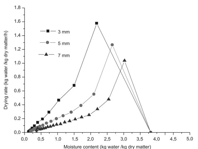
FIGURE 7. The influence of fillet thickness on drying rate (hot air temperature at 45°C, hot air velocity at 2.5 m/s).
