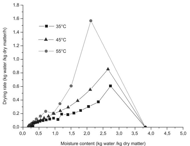
FIGURE 3. The influence of the temperatures of hot air on drying rate (hot air wind speed at 2.5 m/s, fillet thickness at 5 mm).
