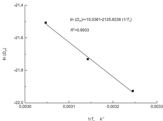
FIGURE 8. Arrhenius-type relationship between effective moisture diffusivity and reciprocal absolute temperature.
