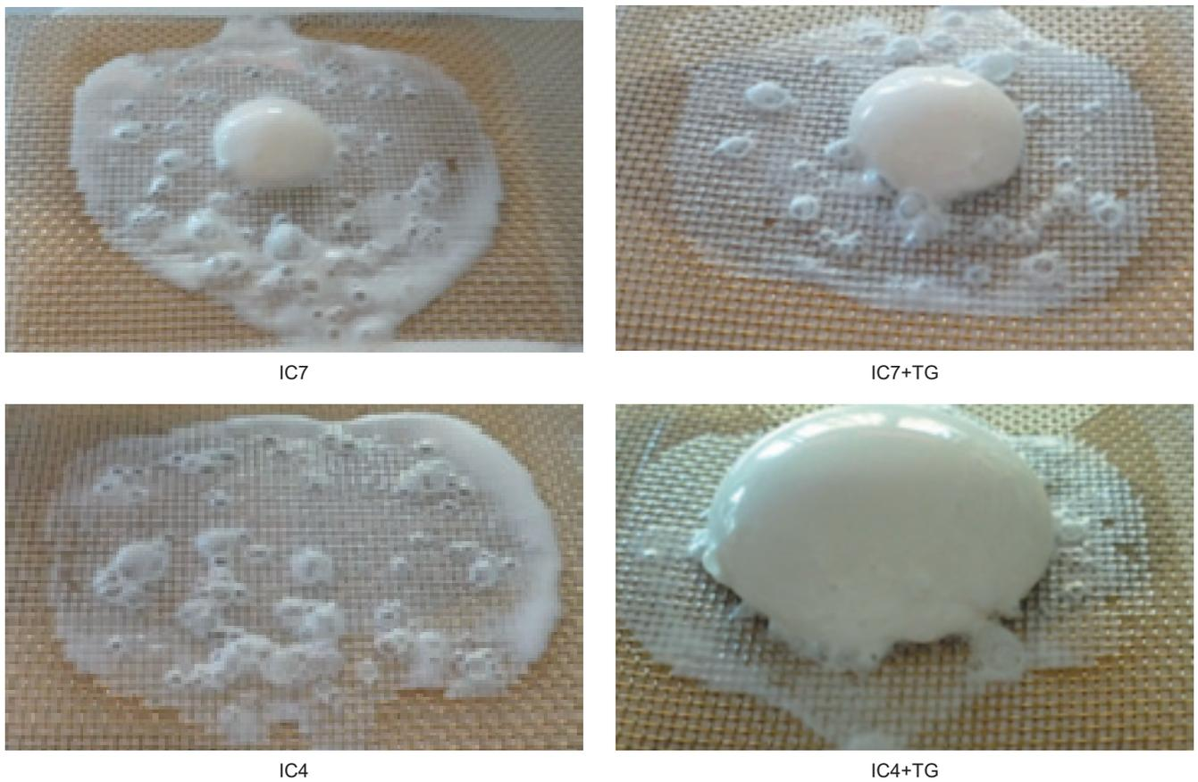
FIGURE 2. Ice cream melting test after repeated thermal shocks (after 120 min) – after 3-month storage.
