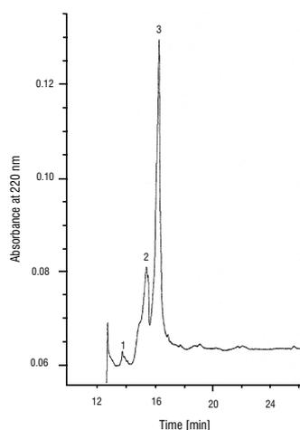
FIGURE 3. EC-SDS electropherogram of rapeseed low molecular proteins.
