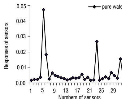
FIGURE 3. Changes in the electric resistance of each chemical sensor in the 32-sensor array of the Cyranose 320 during the investigation of the headspace of pure water.
