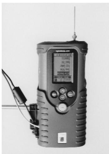
FIGURE 1. The Cyranose 320, The Cyranose 320 Electronic Nose, User's Manual part number 11 60001, CYRANOSciences, Inc.
