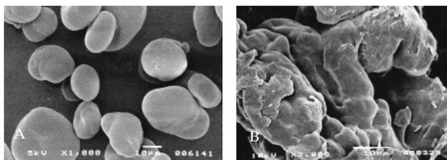
FIGURE 1. Microstructure of native pea starch (A) and its preparation (B).
