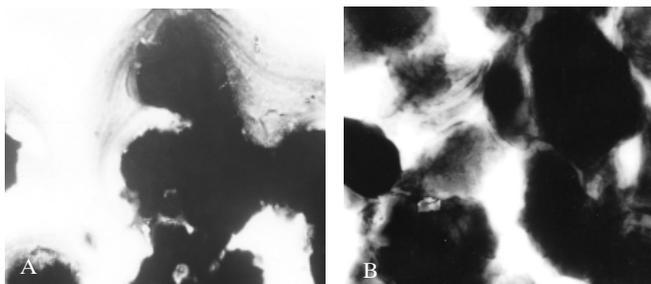
FIGURE 6. Light microscopy of modified pea starch: (a) at 58°C; (b) at 90°C.
