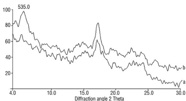
FIGURE 2. X-ray diffraction pattern of pea starch: (a) native, (b) modified.
