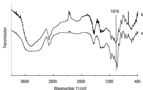
FIGURE 3. FTIR spectra of native and modified pea starch: (a) native, (b) modified.
