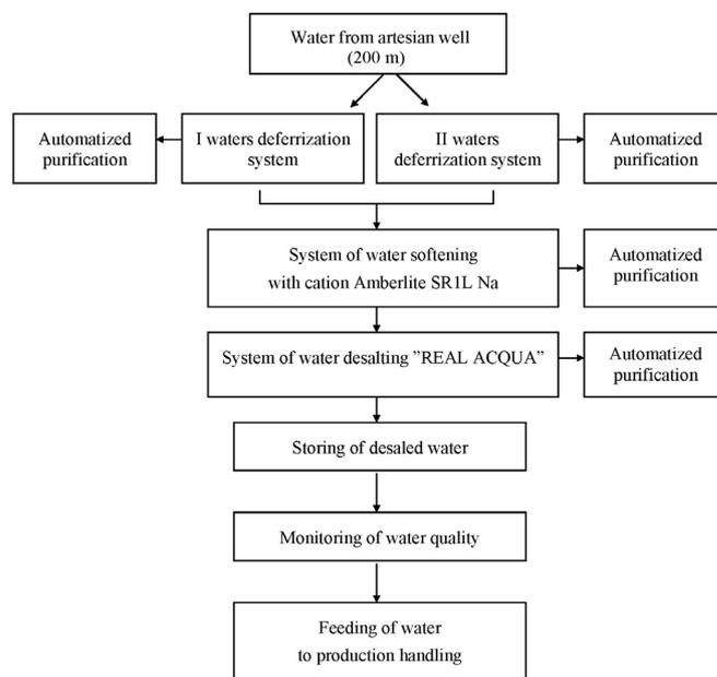
FIGURE 1. Preparation of water of Riga water–pipe for water–ethanol solutions.
