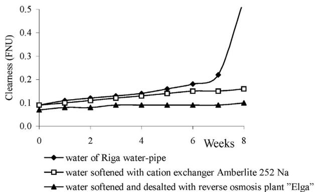
FIGURE 3. Changes in clearness of water–ethanol solutions during storage (water of Riga water–pipe).
