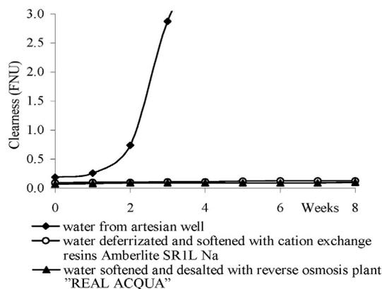
FIGURE 4. Changes in clearness of water–ethanol solutions during storage (water from artesian well).
