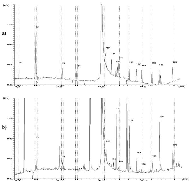
FIGURE 1. GC-ECD chromatograms recorded by Chroma 2001 system (method I): a) standard solution of specified PCB congeners; b) cleaned-up extract of human milk.
