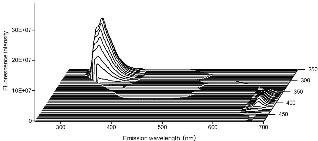
FIGURE 1. The three-dimensional total luminescence spectra of rapeseed oil 2 in n-hexane, 1% v/v.
