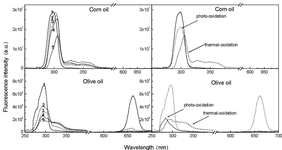
FIGURE 4. Left: Changes in synchronous fluorescence spectra of corn oil (top) and olive oil (bottom) during thermal oxidation, spectra after 1–0, 2–5, 3–10, 4–15, 5–20 h of heating (200°C). Right: Effect of photo- and thermal oxidation on synchronous fluorescence spectra of corn oil (top) and olive oil (bottom).
