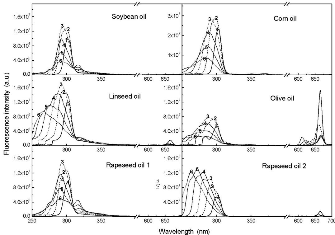
FIGURE 2. Synchronous fluorescence spectra of oils diluted in n-hexane, 1% v/v, recorded at various  $\Delta\lambda$ , 1=10 nm, 2=20 nm, 3=30 nm, 4=40 nm, 5=50 nm, 6=0 nm.
