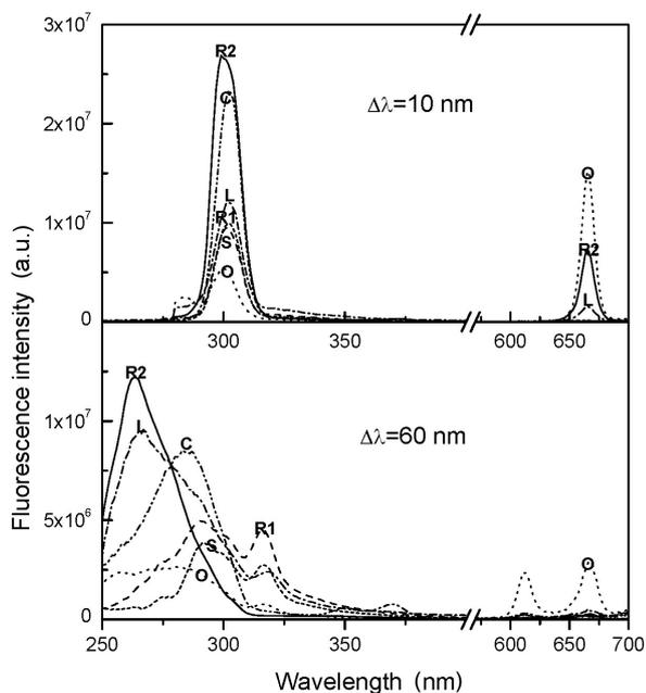
FIGURE 3. Comparison of synchronous fluorescence spectra of oils recorded at  $\Delta\lambda=10$  nm and  $\Delta\lambda=60$  nm: S – soybean oil, O – olive oil, C – corn oil, L – linseed oil, R1 and R2 – rapeseed oils.
