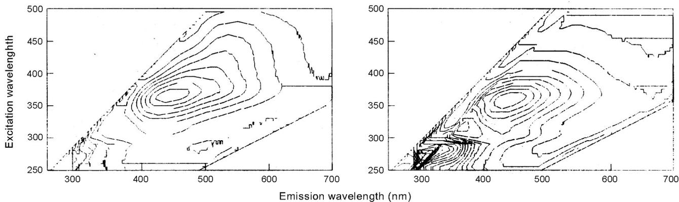
FIGURE 3. Contour maps of total luminescence of undiluted beer 3 stored in a transparent glass bottle in the dark (left panel) and exposed to daylight (right panel).
