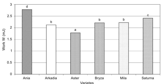
FIGURE 5. The comparison of the work which is needed to obtain the maximum shear stress.
