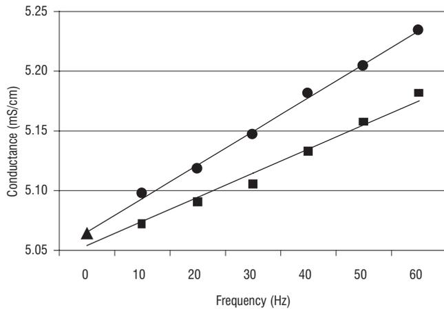
FIGURE 2. Changes in electrical conductivity depending on vibration frequency and time of milk exposure to vibration (■ exposure time 30 min, ● exposure time 120 min, ▲ control sample).
