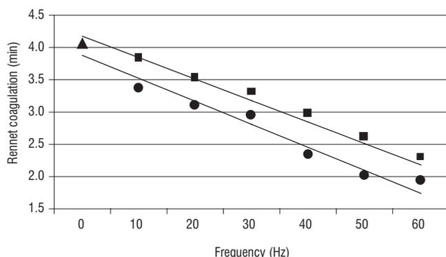
FIGURE 4. Changes in rennet coagulation depending on vibration frequency and time of milk exposure to vibration (■ exposure time 30 min, ● exposure time 120 min, ▲ control sample).
