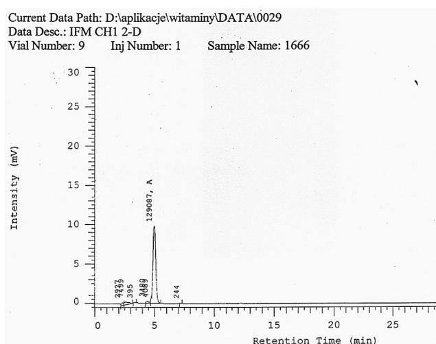
FIGURE 2. HPLC chromatogram for determination of all-trans-retinol (vit. A) in milk.
