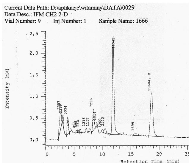
FIGURE 3. HPLC chromatogram for determination of  $\alpha$ -tocopherol (vit. E) in milk.
