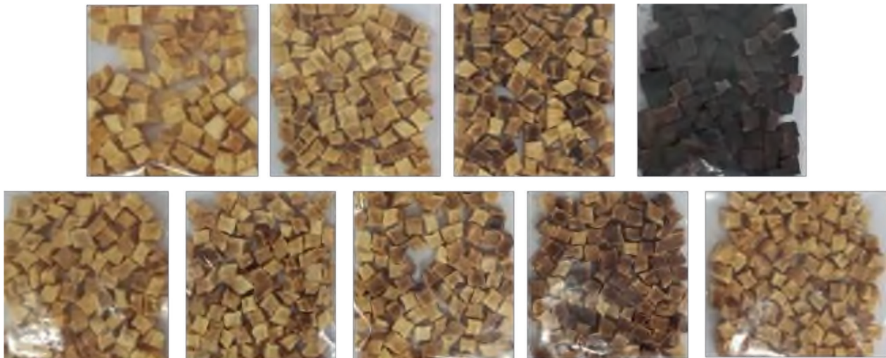
Figure 4. Typical visual appearance of the apple cubes dried using different methods. The four pictures in the first row orderly indicate the hot air-dried sample at 60°C and microwave dried samples at 70, 210, 350 W in a rotary plate microwave dryer (RMD) from left to right. The five pictures in the second row orderly indicate the microwave dried samples at 400; 800; 1,200; 1,600 W in a microwave convection coupled dryer (MCD) and at 1,600 W in MCD with temperature control from left to right.
